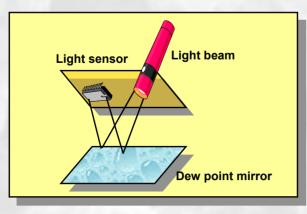
Function : Optical identification of condensation on mirror temperature
